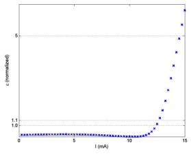
Figure 4: Variation of projected emittance with respect to the beam current.
