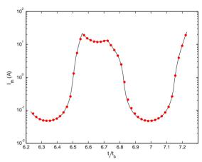
Figure 3: Threshold current obtained by tracking simulation (red dots) and numerical solution (black line) of the dispersion relation Eq. (1).
