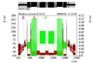
Figure 1: The optics functions of the PEP-X ERL, one recirculation.
