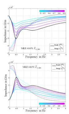
Figure 2: Convergence of the horizontal (top) and vertical (bottom) quadrupolar component to the ultra-relativistic model. The coloured real part (full thick lines) and imaginary part (thin dashed line) are given for different values of  $\beta$ , converging to the black lines given by the ultra-relativistic Tsutsui's model.
