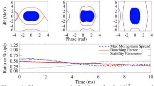
Figure 1: Phase space at 0, 5, 10 ms for  $8 \times 10^{13}$  ppp and evolution of bunching factor, stability parameter (equation 2) and maximum dp/p.
