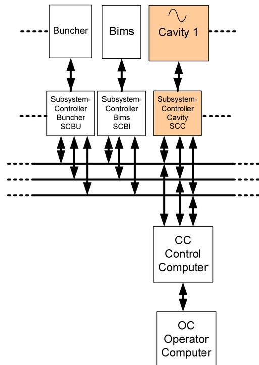
Figure 2: Concept of distributed control system.
