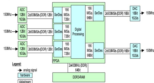
Figure 5: Dataflow on SCCRT.
