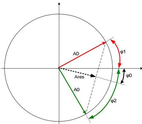
Figure 1: Principle of out phasing control.
