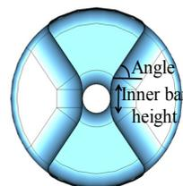
Figure 2: Optimized design parameters of the bars in the parallel-bar geometry.
