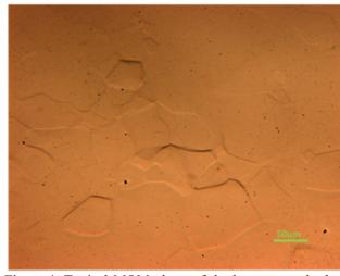
Figure 4: Typical MOM photo of the button sample that shows a Nb removal rate of  $9.7 \mu m/min$ .
