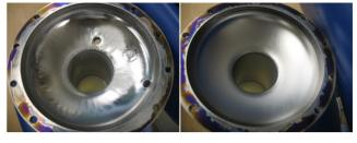
Figure 3: Photos of the demountable cavity after BEP treatment. Left is the upper cell. Right is the lower cell (see text for more details).
