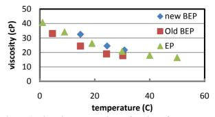
Figure 6: Viscosity measured as a function of temperature for old and new BEP and EP electrolytes.
