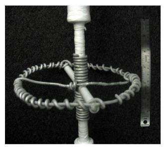
Figure 2: Cathode used in this study.
