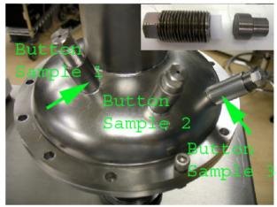
Figure 1: Photo of the demountable cavity fabricated at JLab. The arrows indicate the three button samples. The insert on the upper right corner shows the button sample assembly.
