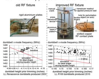
Figure 3: Prevalent frequency errors of past fabrication methods (left) cured by improved tooling (right).
