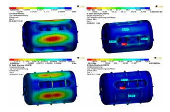
Figure 3: Deformation and max. von-Mises stress of the cavity due to evacuation without stiffening ribs (top) and with stiffening ribs (bottom)0
