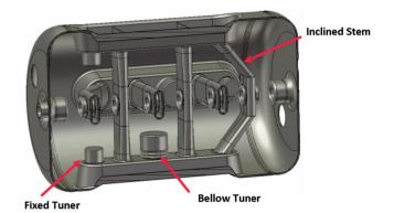
Figure 1: Layout of the sc 325 MHz CH cavity [4].
