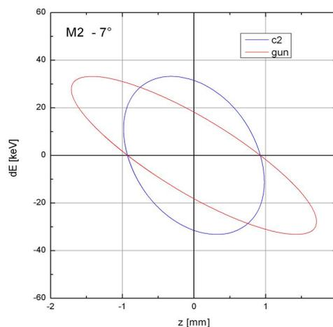
Figure 6: an example of the longitudinal phase space at the exit of the gun cavity with laser phase  $-7^\circ$  (red).
