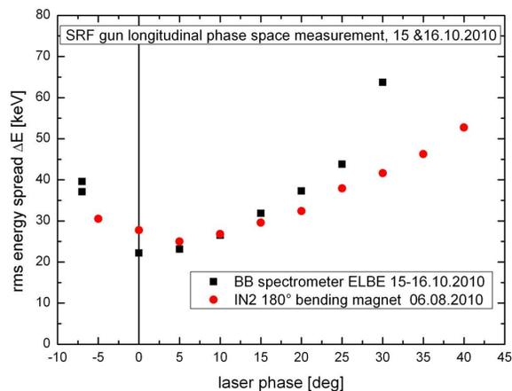
Figure 4: measured curves of the rms energy spread versus the gun phase. The red dots give out the measurement results from the gun diagnostic beam line and the black squares show the result with BB spectrometer in the ELBE beam line.
