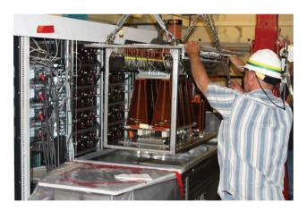
Figure 3: Final modifications to ScandiNova K2-3X high voltage modulator.
