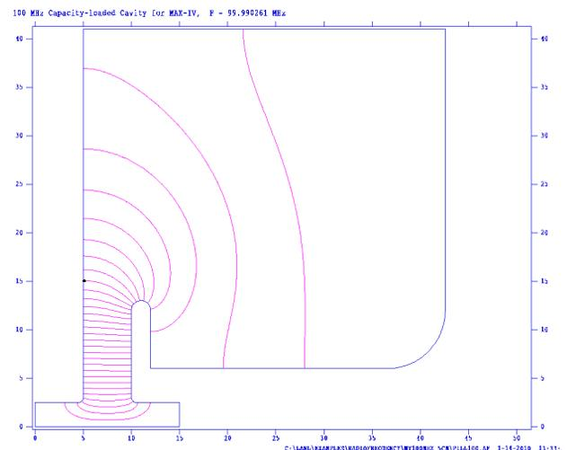
Figure 1: Main cavity profile.
