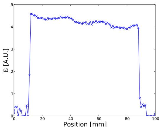
Figure 3: Longitudinal scan for a mode at 319MHz.
