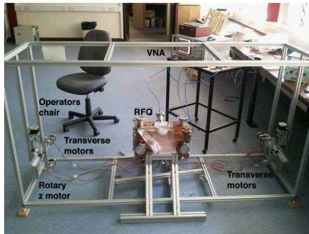
Figure 1: Existing bead-pull setup.
