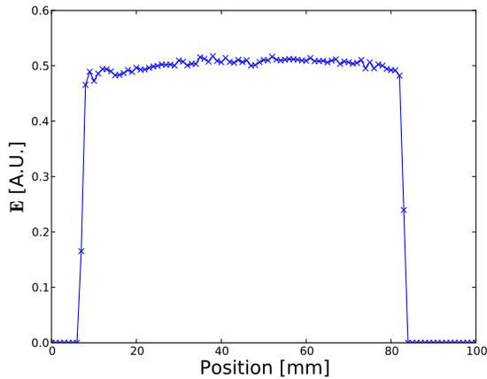
Figure 6: Longitudinal scan for a mode at 328MHz.
