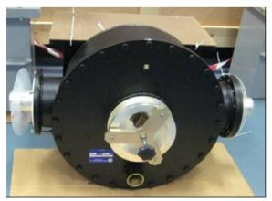
Figure 3: CaCo, a Cavity Combiner.
