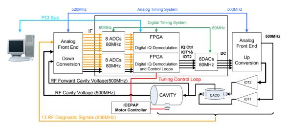
Figure 5: Digital LLRF Hardware Scheme.
