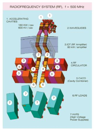
Figure 1: Two RF plants in one straight section.
