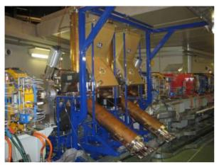
Figure 2: Two Dampy cavities installed in the tunnel.
