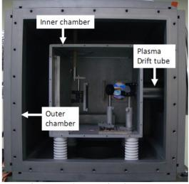
Figure 1: LIS target chamber at IMP
