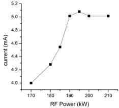
Figure 9: Beam current from RFQ vs. RF power of RFQ
