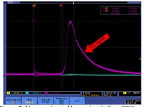
Figure 7: Non-accelerated beam signals from FFC and FCT
