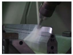
Figure 4: Vane-tip machining of an aluminum test segment with the ball-end mill.
