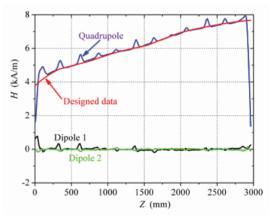
Figure 10: Field distribution of the quadrupole and dipole modes after the pre-braze tuning.
