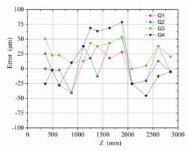
Figure 7: Measurement result of the vane-tip gaps at the position of the tuners and vacuum ports.
