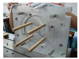
Figure 9: The dipole stabilizer rods.
