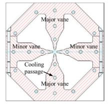
Figure 1: Cross section of the first segment at a fixed longitudinal position.
