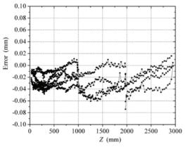
Figure 5: CMM result for the vane-tip height vs. *z* of all the vanes.
