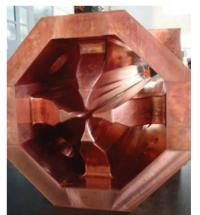
Figure 6: Assembled first segment of the CPHS RFQ.
