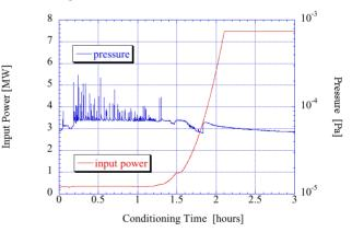
Figure 5: Input power and vacuum pressure history of RF conditioning of prototype isolator (normal direction).
