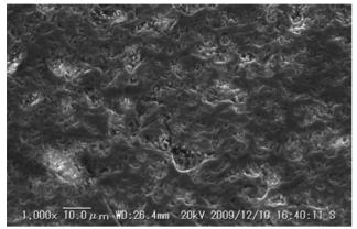
Figure 2: SEM image of a garnet-ferrite surface.
