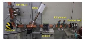
Figure 4: Prototype vacuum isolator (above: a viewport is located to observe ferrite surface) and setup for a high power test (below).
