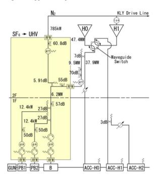
Figure 1: Waveguide system for injector section of SPring-8 linac.
