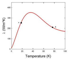
Figure 1: Thermal conductivity of molybdenum: point "A" normal operation, point "B" for cavity conditioning.
