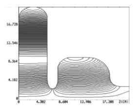
Figure 5: Electrical field lines in the gun cavity with a TM020 mode in the half cell and TM010 mode in the full cell. The vertical axis is the cavity radius; the horizontal axis is the cavity length.
