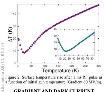
Figure 2: Surface temperature rise after 1 ms RF pulse as a function of initial gun temperature (Gradient 60 MV/m).
