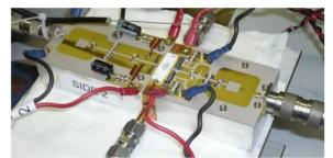
Figure 10: RF module using printed balun transformers.
