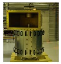
Figure 8: Lab prototype with the output coupler.
