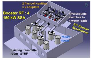
Figure 5: Four SSA replacing the klystron on the booster.
