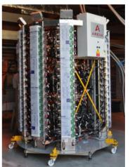
Figure 2: First 75 kW amplifier tower combining 128 RF modules.
