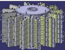
Figure 7: Cavity combiner with 22 pallets, each integrating 6 RF modules and their power supplies.
