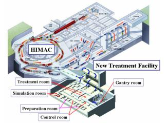
Figure 2. Layout of HIMAC and new treatment research facility. Treatments with the pencil-beam 3D rescanning have been successfully carried out at one fixed port room in the new treatment facility, since May 2011.
