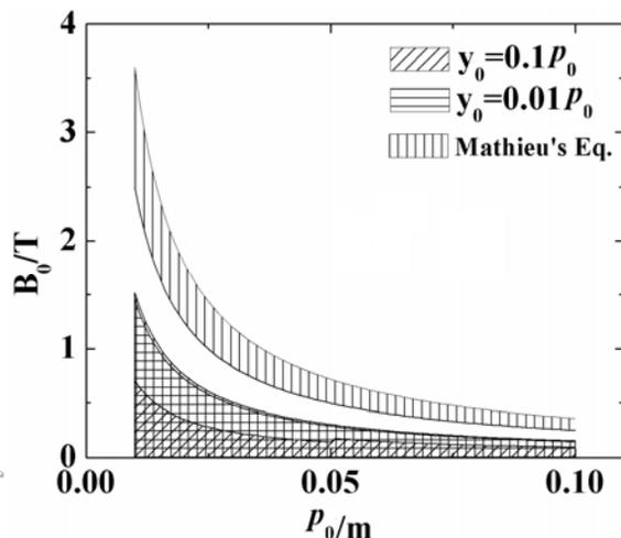
Figure 3: The stable regions predicted by the Mathieu's Equation and the numerical calculations.
