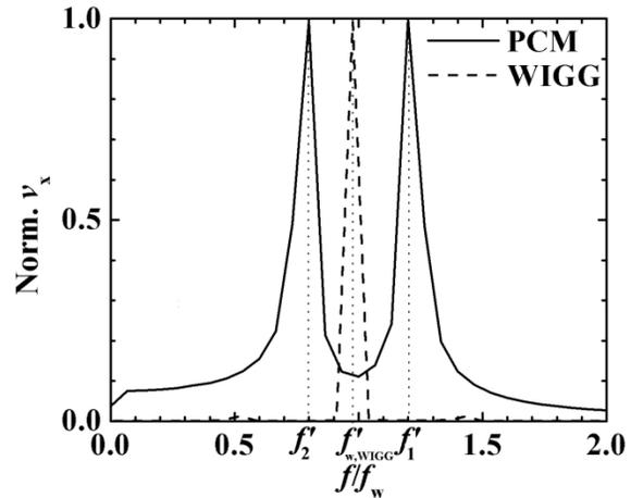
Figure 2: FFT of the curves of the transverse velocities  $v_{x,PCM}/v_{z0}$  and  $v_{x,WIGG}/v_{z0}$  for the case  $B_0 = 0.2T$  and  $p_0 = 2\text{cm}$ .
