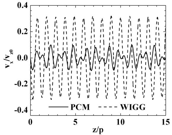
Figure 1: Normalized transverse velocities  $v_{x,PCM}/v_{z0}$  and  $v_{x,WIGG}/v_{z0}$  versus axial position  $z/p_0$  for the case  $B_0 = 0.2T$  and  $p_0 = 2\text{cm}$ .
