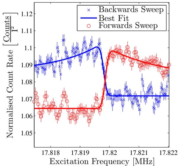
Figure 2: Resonant spin depolarisation at spin tune.
