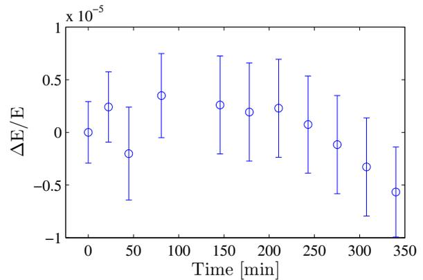
Figure 3: Energy drift with time.
