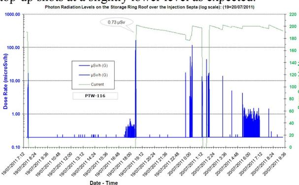
Figure 8: Photon radiation levels above the injection point including a top-up test.
