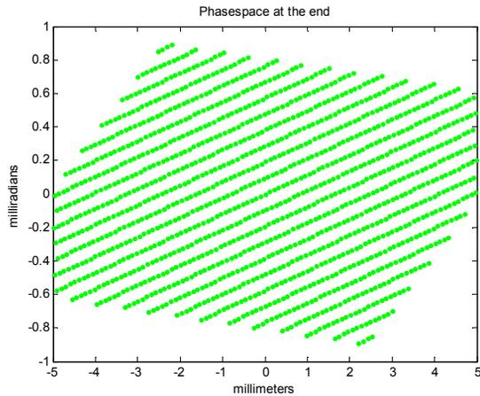
Figure 3: Electron distribution in horizontal phase space at the end of the transfer line.
