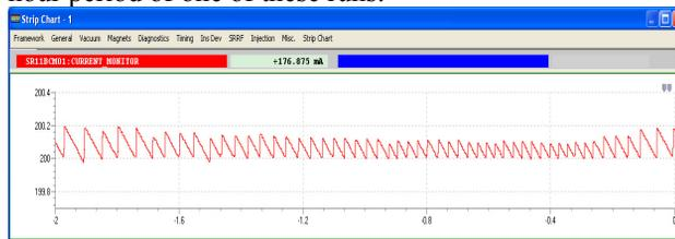
Figure 1: Current during a top-up run.
