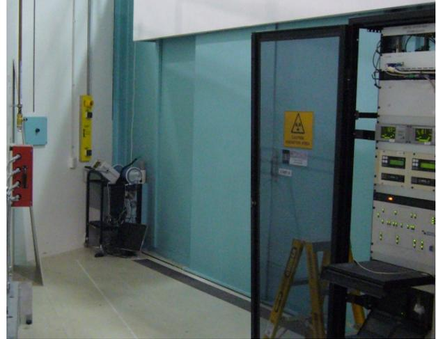
Figure 5: Photon radiation monitor next to the first optical enclosure.
