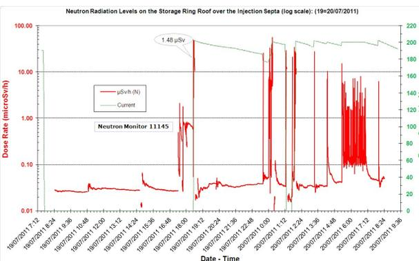
Figure 9: Neutron radiation levels above the injection point including a top-up test.
