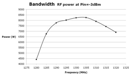
Figure 10: Bandwidth of the SSPA
