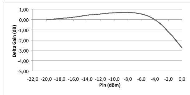
Figure 7: Gain deviation of the SSPA
