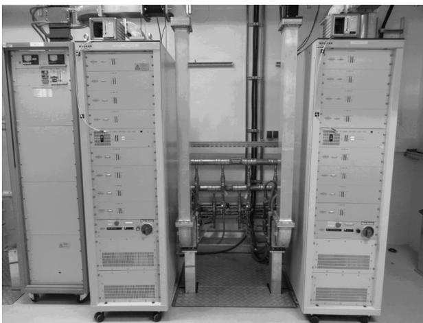
Figure 4: 10 kW SSPA (BRUKER)
