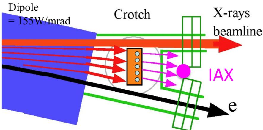
a tiny fraction ( $\sim 2 \cdot 10^{-6} = 300\mu\text{W}/\text{mrad}$ ) traverses the crotch : Xrays > 150KeV
