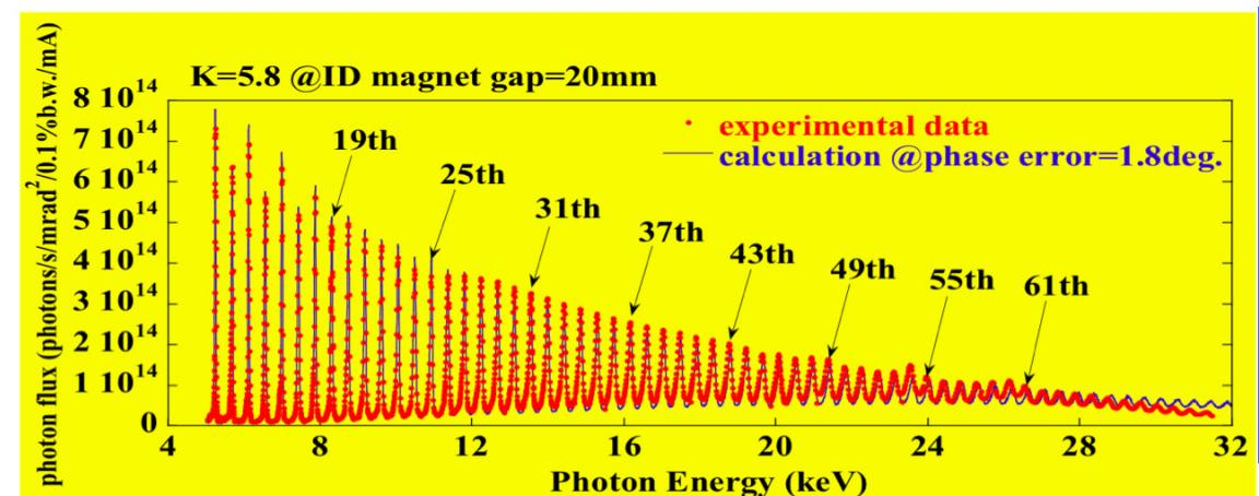
Elaborate tuning of the magnetic field has led to the rms phase error < 2 degrees, which allows us to observe many clear peaks of the higher harmonics.
