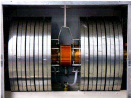
High-gradient magnetic alloy loaded bunch compressor cavities
