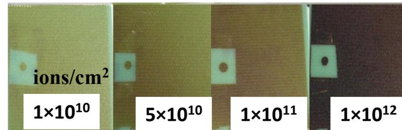
**$10^{12}$  heavy ions make the same damage as  $10^{16}$  protons in organic insulators.**
