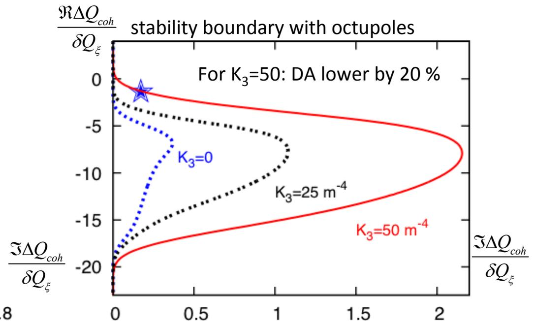
**Octupoles in combination with space charge can be used for the stabilization of dc and head-tail instabilities in SIS-100.**
