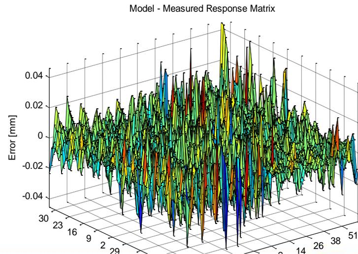
Difference between the measured and the model response matrices with LOCO
