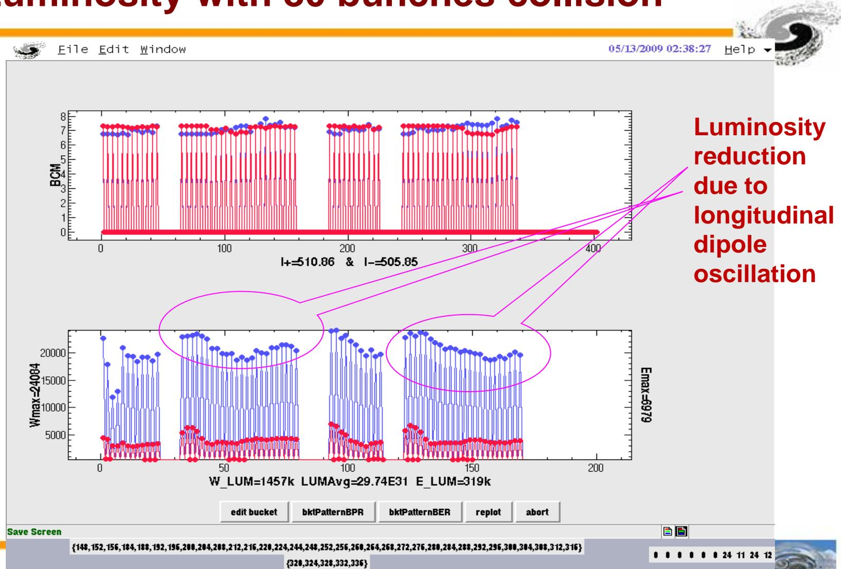
Luminosity reduction due to longitudinal dipole oscillation
