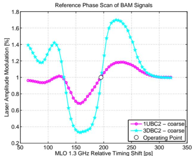
Shift 1.3 GHz phase of reference laser pulse to sample RF pick-up signal
