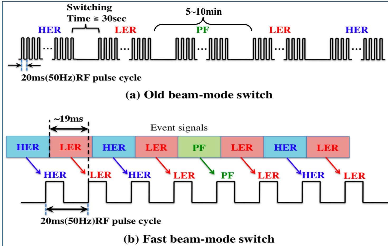
Schematic view of the beam-mode switches.
