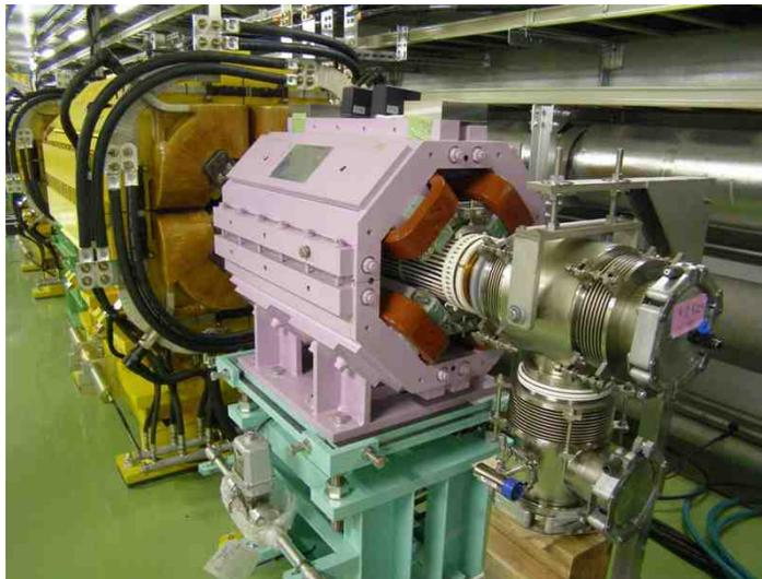
EQ: for constant spill structure ( $< 100$  Hz)
