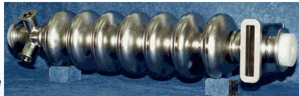
KEK ERL 9-cell cavity (1.3GHz) with beam pipe HOM absorber.
