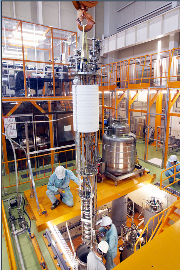
Vertical Dewar test for gradient performance check. (KEK-STF as an example)
