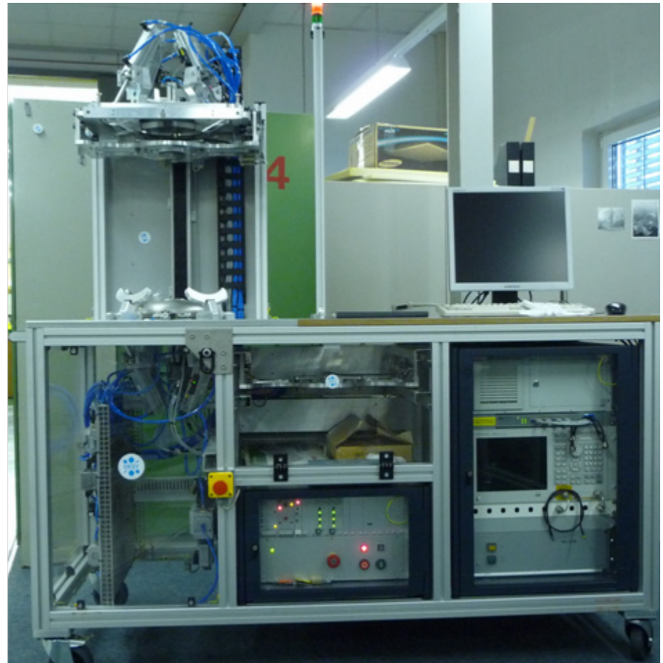
Equipments for RF measurement of half cells, dumb bells and end groups (HAZEMEMA)
