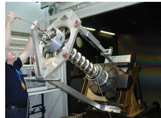
EB welding of joint 1, 2
