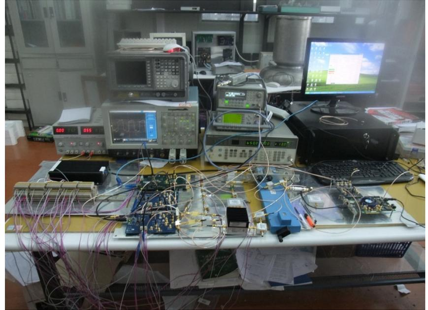
**The LLRF loops based on FPGA is under test**
