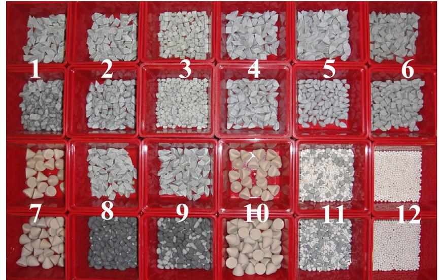
Due to the EBW problem, we made 12 times CBP on this cavity with different abrasives ( $\text{SiC}$ ,  $\text{Al}_2\text{O}_3$ ), bonders (ceramic and plastic), stone shapes and filling amount. The rotation speed around the cavity axis was 100 - 150 rpm, and 100 rpm around the machine axis. It took about 62 hours to totally remove **190  $\mu\text{m}$**  of the equator wall thickness.
