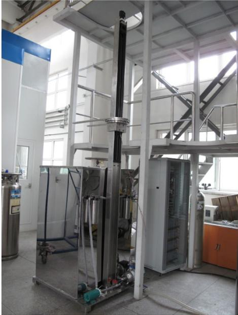
Ultrasonic cleaner for the 9-cell cavity
