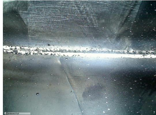
Many sputters were found in the equator area of cell#2 to cell#8. We are still investigating the reason of sputtering. The EBW vendor is expected to be qualified because they made the IHEP 40 MV/m single cell CP cavity.
