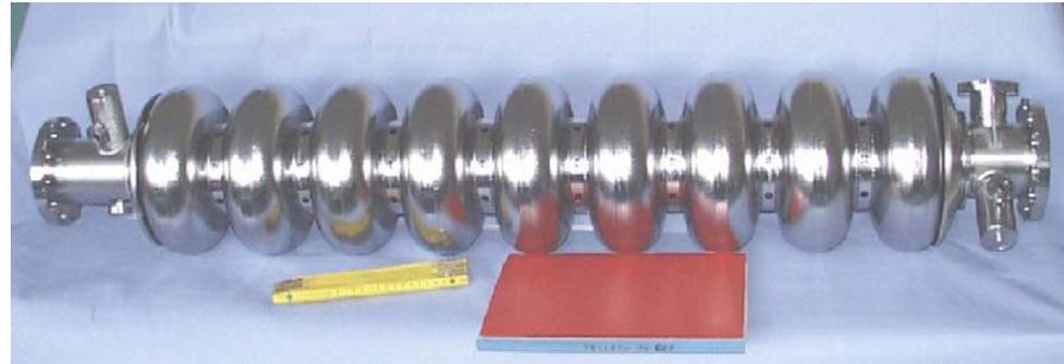
More than 75 cavities with gradients up to **35 MV/m**
