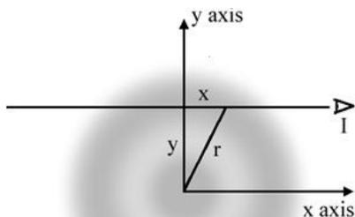
Figure 2: Schematic of the cylindrical symmetry of a discharge.
