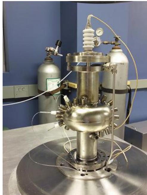
Figure 1: Multiple optical fiber set-up for single cell cavity.
