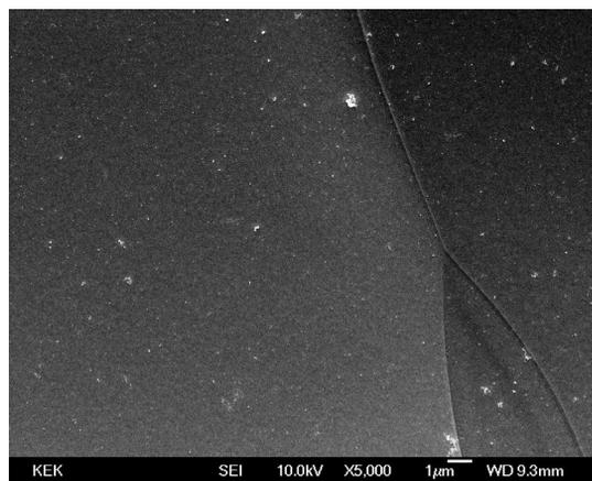
Figure 7: SEM image of the stained area of the niobium sample. Many dots were found in both of the non-stained and stained area.
