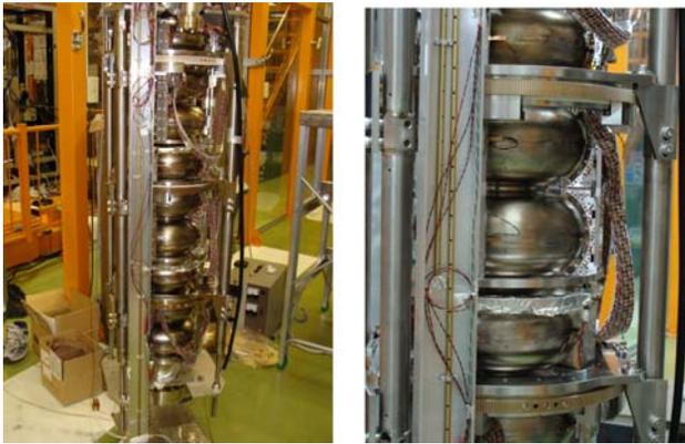
Figure 2: Setup of a 9-cell cavity for the vertical test with a rotating mapping system.
