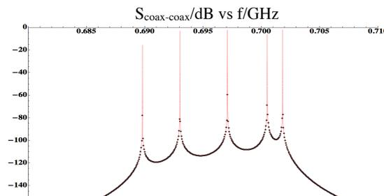
Figure 5: Detail of the pole fitting result (red line) for the fundamental mode passband.
