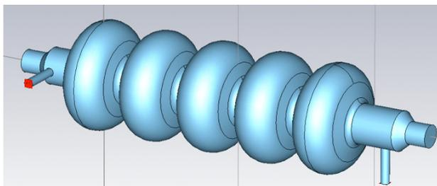
Figure 1a: Computation model of the SPL- $\beta=1$ -cavity, equipped with shortened outer beam pipes of 40 mm radius and with two coaxial HOM coupler without fundamental mode filters (comp. Figure 1b).
