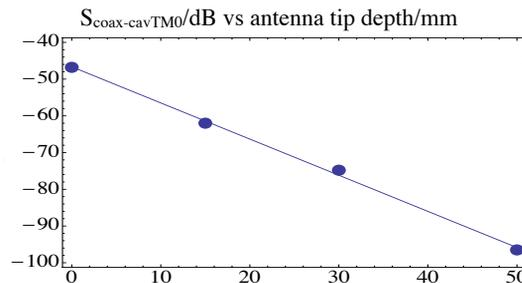
Figure 6: Transmission of the coax-cavity transition, computed as coax- $TM_0$  scattering parameter at 704.4 MHz for different antenna tip distances, measured from the beam pipe outer radius. Blue dots are numerically calculated, straight line is the best linear fit.
