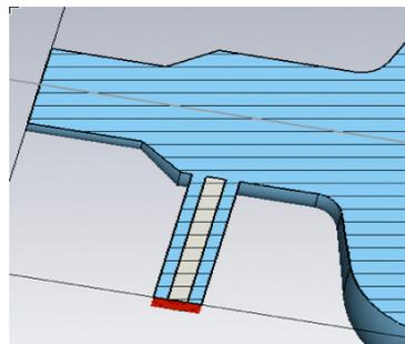
Figure 1b: Cross section of the coaxial HOM coupler, shown with an antenna tip of the inner conductor (light grey) on beam pipe radius. In order to adjust the fundamental mode loading the length of the inner conductor may be reduced if damping of higher order modes is kept strong enough.
