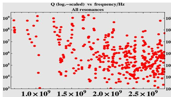
Figure 4: Q value distribution of the SPL-cavity with coaxial couplers as shown in Figure 1, computed with the pole fitting algorithm. The fundamental mode (belonging to the leftmost groups of dots) reaches almost exactly  $Q=10^8$ , which is coupled by far too strongly.
