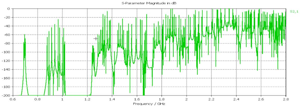
Figure 2: Transmission spectrum computed with the "FastResonant" solver of CSTStudio© [4] for the setup shown in Figure 1, using an antenna tip depth of 0. It contains more than 400 resonances with widely spread Q-values.
