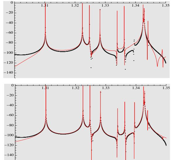
Figure 3: Pole fitting (red lines) applied on a small fraction of the spectrum (dots given as  $S_{\text{coax-coax}}(f/\text{GHz})$  in dB) shown in Figure 2. Original (upper plot) and improved procedure. The deviations at the spectrum's limits are due to the neighbouring poles, here missing.
