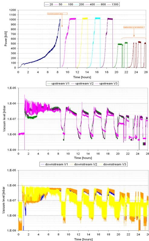
Figure 2: RF conditioning results for 2 pairs of TTF3 FPC conditioned in series.
