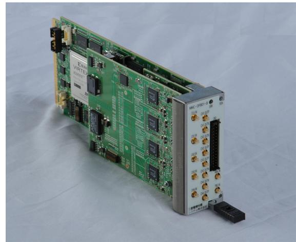
Figure 1: Virtex-5-based MicroTCA card (embedded IOC) for the digital RF feedback control
