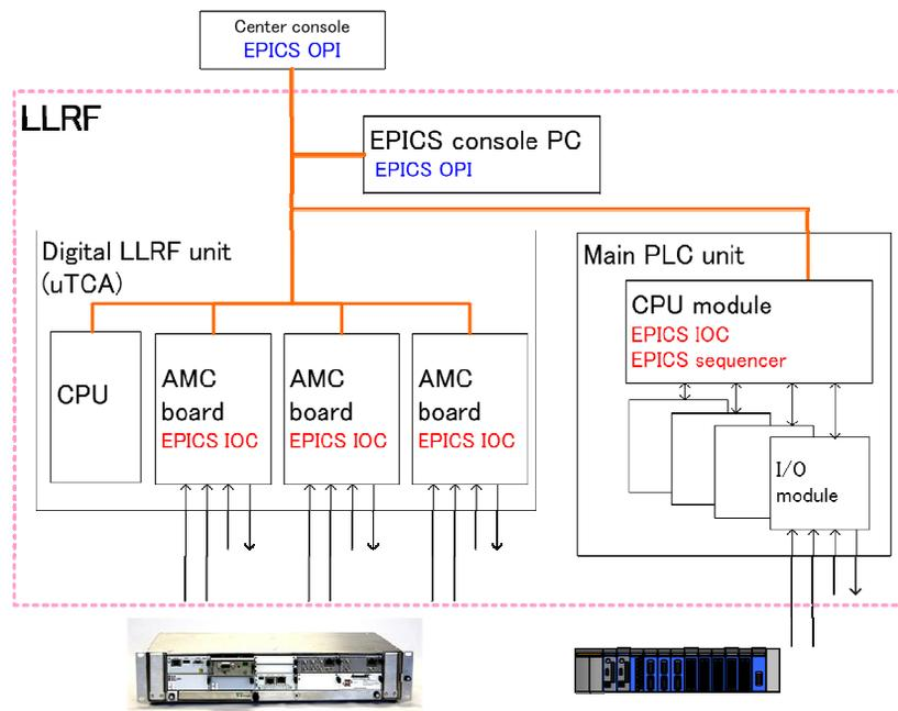
Figure 2: Configuration of the new LLRF control subsystem.
