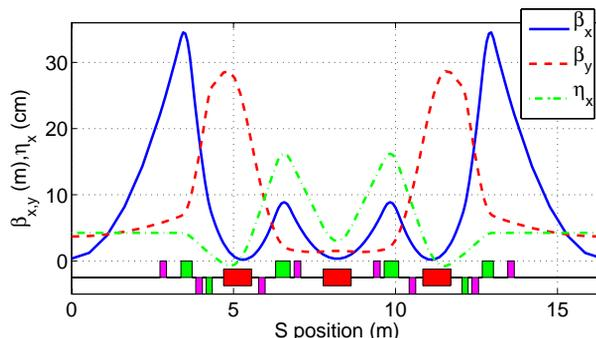
Figure 1: A low- $\beta$  lattice of one of 12 sectors for ALS upgrade. The working tunes are  $\nu_x = 1.81$  and  $\nu_y = 1.77$ . The lattice is optimized for the brightness at insertion devices.
