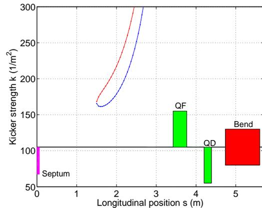
Figure 4: Pulsed sextupole injection matching for the ALS low- $\beta$  lattice. A 1 meter long pulsed sextupole kicker is located at 1.5 m away from the septum. The mismatch and match injections are represented by the red and blue color, respectively.
