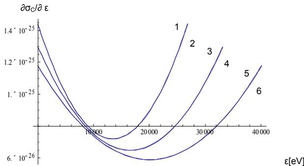
Figure 2. Compton cross section vs radiated photon energy calculated with quantum approach (1-  $E_0=38.7$  MeV, 3-  $E_0=43$  MeV, 5-  $E_0=47.3$  MeV) and classical electrodynamics approach (2 -  $E_0=38.7$  MeV, 4 - 43 MeV, 6 - 47.3 MeV).
