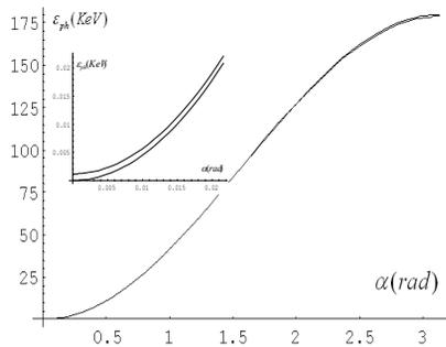
Figure 1. The energy of the first harmonic of scattered radiation depending on interaction angle ( $E_0=100$  MeV).
