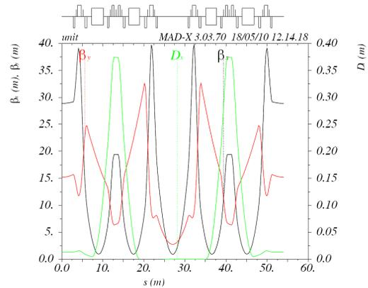
Figure 1: Lattice functions for 18 period DDDBA lattice
