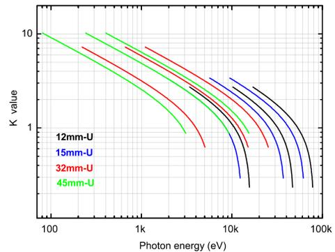
Figure 5: Undulator strength vs. photon energy of TAC undulators
