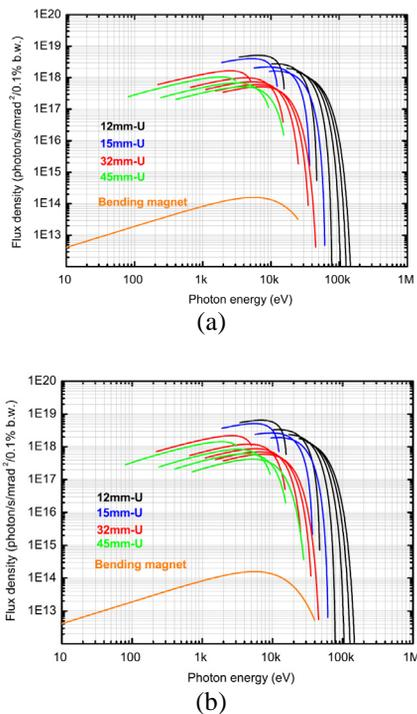
Figure 6: Flux density of the synchrotron radiation from IDs: a) no DWs, b) with DWs.
