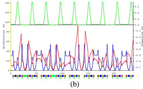
Figure 4: Lattice functions: a) no DWs and IDs, b) with DWs and IDs.
