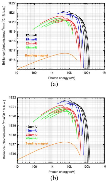
Figure 7: Brilliance of synchrotron radiation emitted from the undulators at the TAC storage ring: a) no DWs, b) with DWs.
