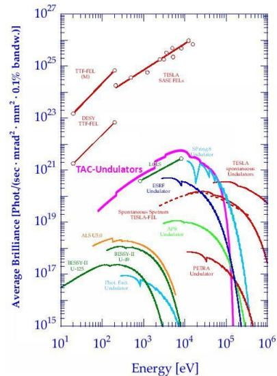
Figure 8: Comparison of TAC undulators with SR sources at the world.
