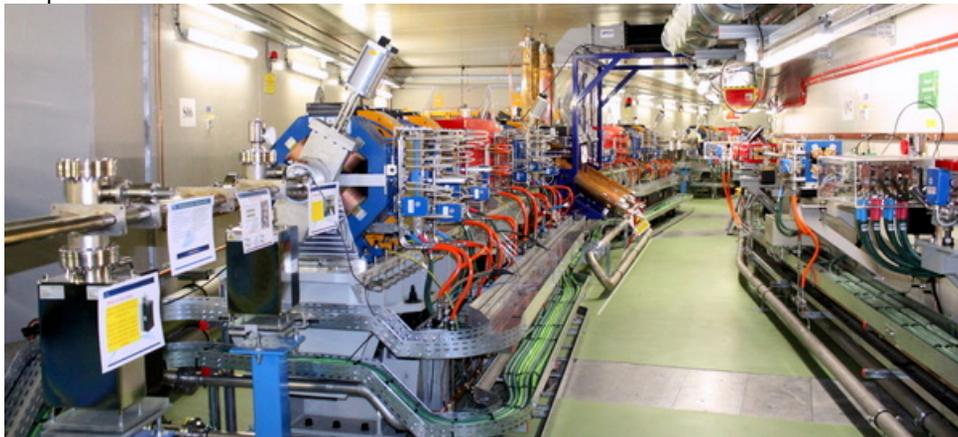
Figure 1: View of the tunnel, with the booster synchrotron in the right and the storage ring in the left.
