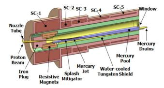
Figure 1: Concept of a 4-MW target station based on a freemercury jet inside at 20-T solenoid. Both the proton beam and the mercury jet are tilted with respect to the magnet axis to maximize collection of low-energy pions. The mercury is collected in a pool that serves as the proton beam dump.
