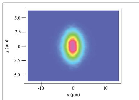
Figure 2: Interaction point spot size of the muon beam whose properties are given in Table 2. The quadrupole gradient is 990 T/m.
