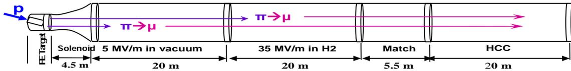
Figure 1: Layout showing modified tapered solenoid ending with  $B_z=4.2T$ , 20 m of RF with 5 MV/m in vacuum, 20 m of RF with 35 MV/m in H<sub>2</sub> gas and Be windows with varying thicknesses, the matching section, and the HCC.
