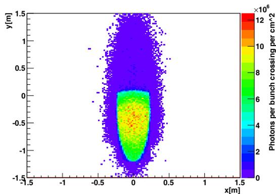
Figure 2: Photons backscattered from the intermediate dump (observed at the upstream end of the dump, 67 m from the IP). The area of higher photon density corresponds to the asymmetric aperture in the dump.
