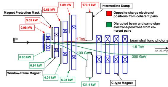
Figure 1: Schematic layout of the CLIC post-collision line showing the power losses at the magnet absorbers and intermediate dump.
