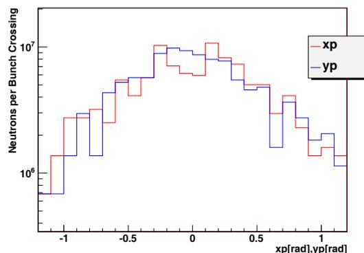
Figure 6: Horizontal and vertical angular distribution of backscattered neutrons, obtained from GEANT4 simulations at the upstream (entrance) end of the CLIC main beam dump.
