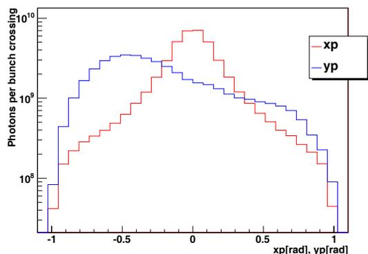
Figure 5: Angular distribution of backscattered photons (as Figure 2, observed at 67 m from the IP).
