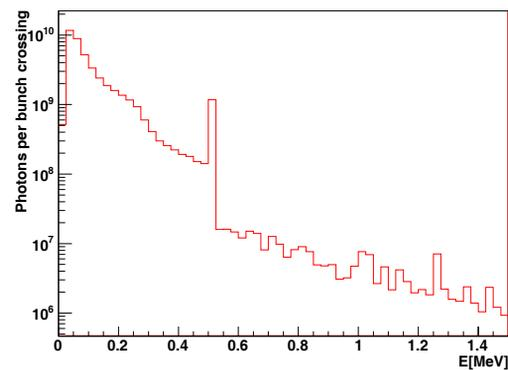
Figure 4: Energy distribution of backscattered photons (as Figure 2, observed at 67 m from the IP).
