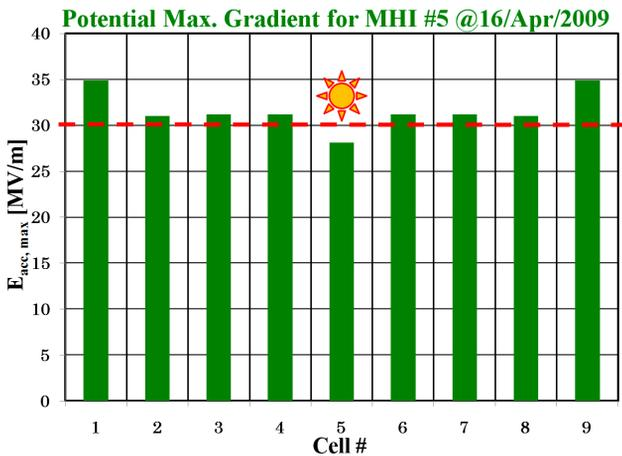
Figure 3: Table of pass-band measurement and potentially maximum gradient for each cell.
