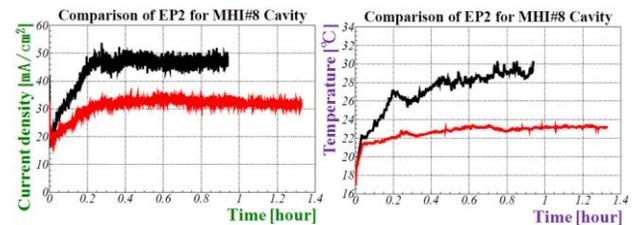
Figure 1: Comparison of EP parameters between the different conditions. Left shows the time trend of the current density ( $\text{mA}/\text{cm}^2$ ) and right shows the temperature ( $^\circ\text{C}$ ) of the EP acid inside the cavity.
