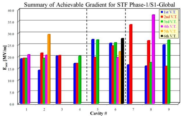
Figure 2: Final result of vertical tests for S1-Global.
