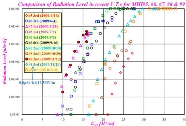
Figure 4: Radiation level measured on top flange of cryostat.
