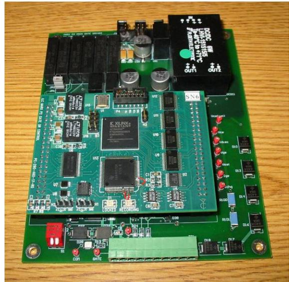
Figure 2: Photograph of the gate driver designed to control 6.5 kV IGBTs in the main stage. The digital control board is stacked to the gate driver board. Dimensions of the gate driver board and the digital control board are 4.5"×5.5" and 3.3"×2.5", respectively.
