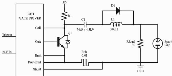
Figure 3: Circuit schematic of the test setup used to evaluate the effectiveness of the designed gate drivers. Values for resistor *Rload* and inductor *L1* are based on the design of the Marx cell PEBB.
