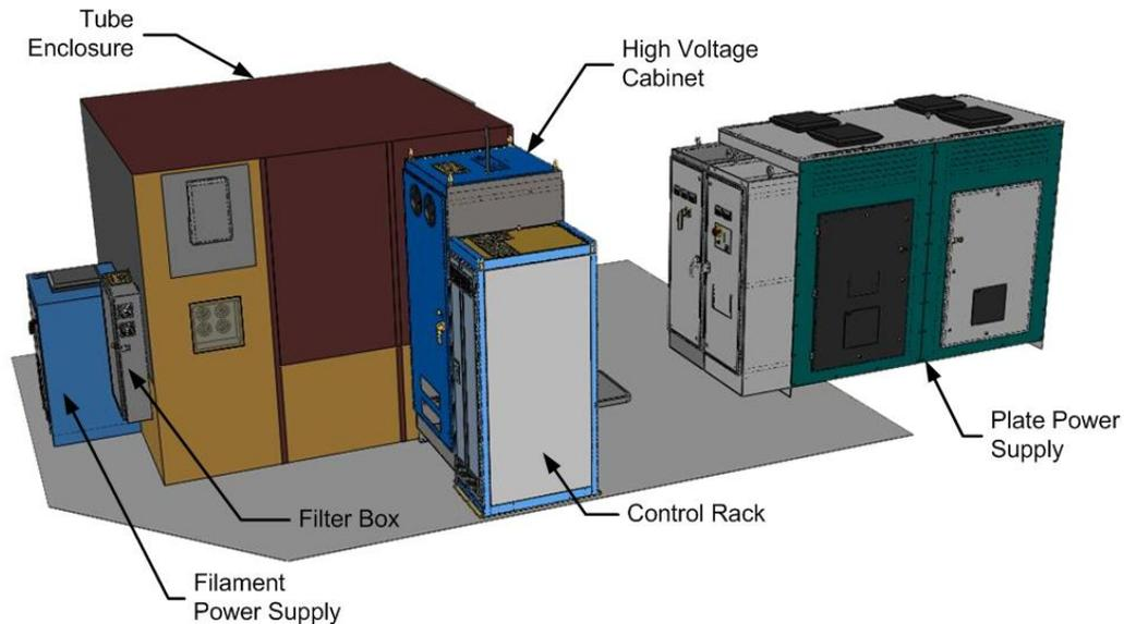
Figure 2: Tetrode test stand assembly.
