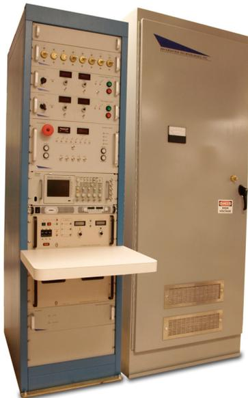
Figure 3: The control rack and high voltage cabinet of the tetrode test stand.
