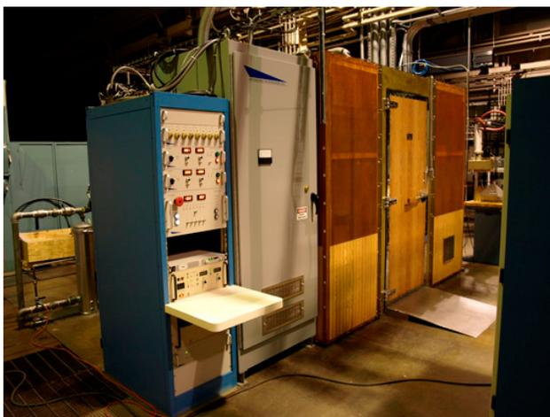
Figure 1: Tetrode Test Stand installed at Burle Industries.
